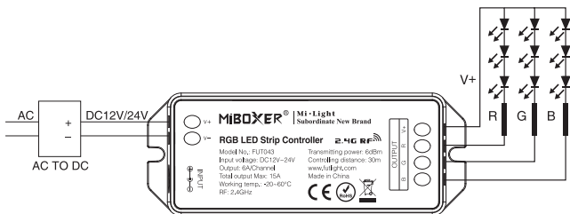
Controller connect to RGB LED strip diagram
